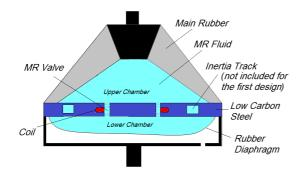
Fig. 2. Schematic of the MR engine mount
