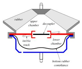
Fig. 1. Schematic of a passive hydraulic engine mount
