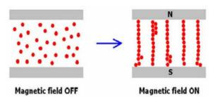
Fig. 3. MR fluid with and without magnetic field
