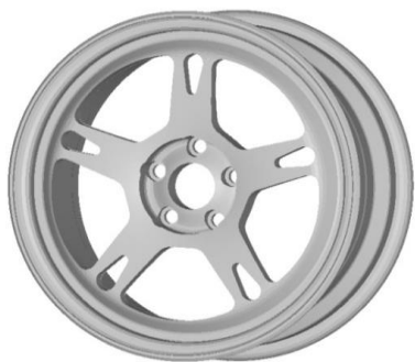
Figure 20: The optimized design after topology optimization
