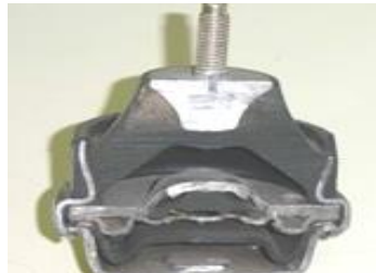
Fig24. Hydraulic engine mount with Inertia track
