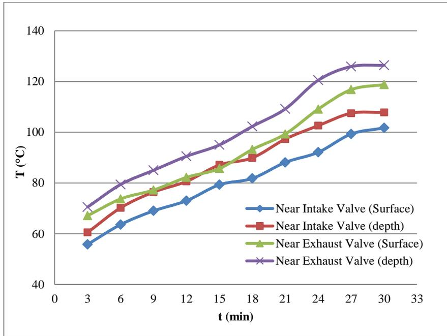
Fig.6. Valve Cover Transient Temperature in 4000 rpm
