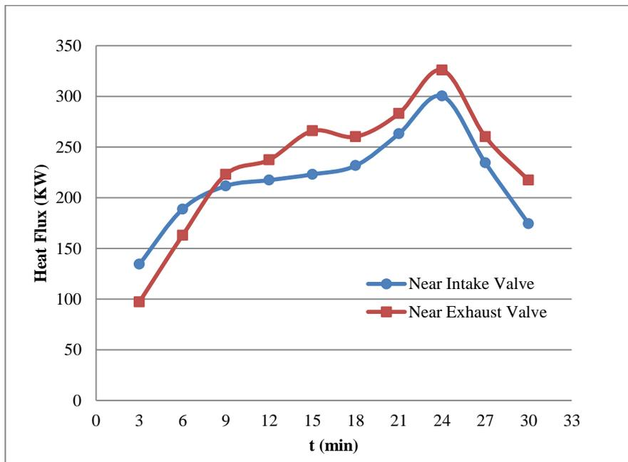
Fig.7. Valve Cover Transient Heat Flux in 4000 rpm
