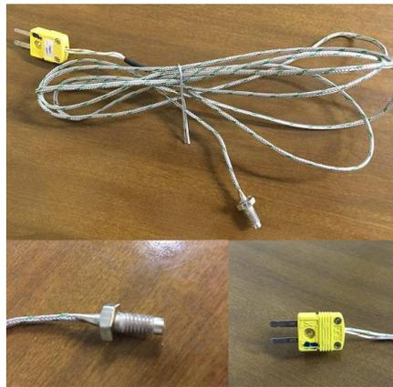
**Fig1..** Sample Thermocouple and Its Sensor and Socket
