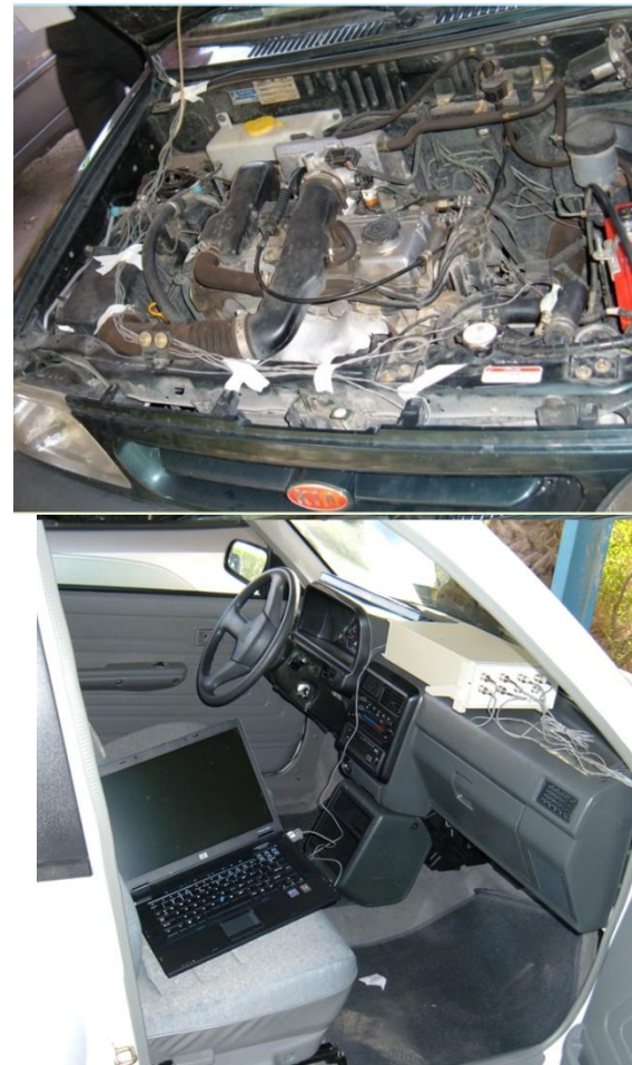
Figure 7: The data acquisition system and temperature sensors
