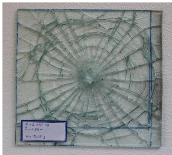
Fig12. .specimen after test code D-B-T-5
